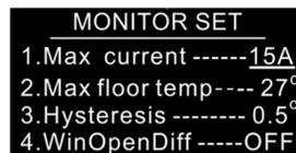
Short press button to select the item would like to modify, then short press move up and move down buttons to modify value of selected item, then short press button **F** to save and quit, short pressing button only quits without saving.
