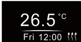
If the device operation mode is set to any other mode except OFF Mode, and there is no operation within 2 minutes, the device will go to this standby interface.
