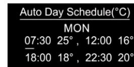
On Auto Day Schedule interface, short press button to select the time or temperature that you would like to modify, then short press move up and move down buttons to modify value, then short press button **F** to save and quit, short pressing button only quits without saving.
