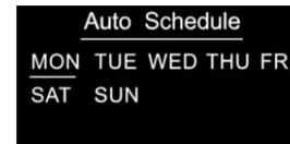
**Schedule setting method 2:** on System Setting Interface, meanwhile the device is under Auto Mode , short press button to enter into Auto Mode Schedule weekly setting interface quickly:
