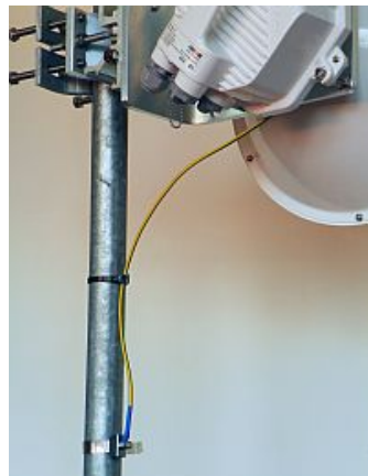
Fig. 4.10: Grounding the RAY unit
