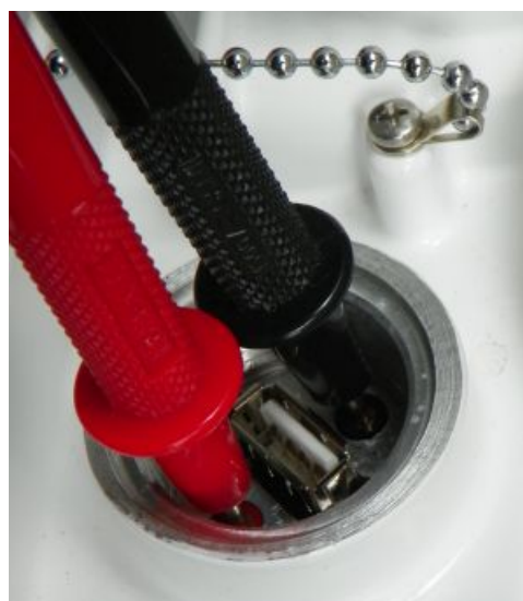
Fig. 1.15: RSS voltage contacts
