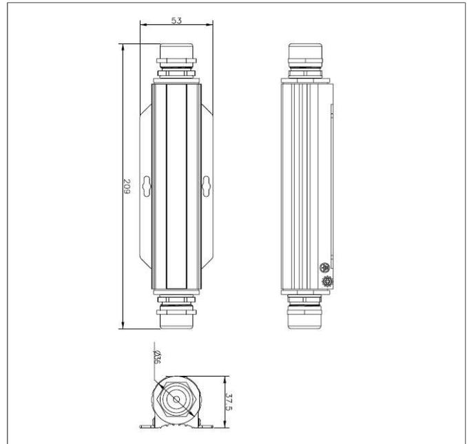
**Order Info.** PT-PR01G-OT 44-57Vdc(Max 60Vdc)/100W/1000Mbps/10KV Surge Protection/IP67/outdoor use
