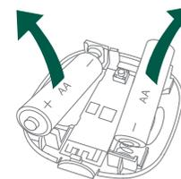
2. Replace the batteries respecting the polarities.
