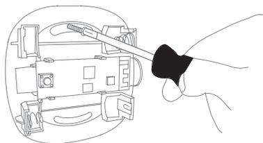
3. Insert batteries respecting the polarities.
