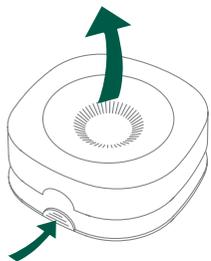
2. Insert two AA batteries respecting the polarities.
